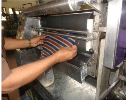
Plate 6. Application of Palmarosa oil microcapsules on organic cotton knit fabric through pad dry cure method
