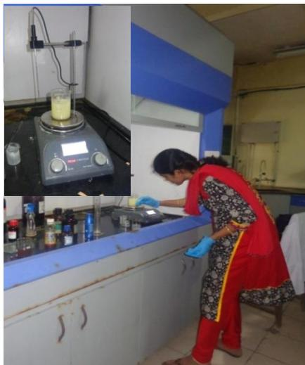
Plate 4. Preparation of Plamarosa oil microcapsules through Interfacial polymerization technique
